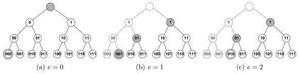
Here, r = 3, and the first 3 epochs are shown. A double circle indicates the identity used for encryption in the current epoch, and shaded circles indicate state that the BTE scheme retains during that epoch.
