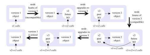
**Fig. 3.** The interceptor approach, presented as a sequence of states of a node. Large arrows are state transitions. In each state, the box is the current object, and the circles are SOs. Objects may delegate calls as indicated by the small arrows. One object in each state intercepts all calls.
