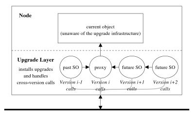
Fig. 1. The structure of a node.
