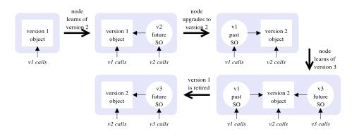
**Fig. 2.** The direct approach, presented as a sequence of states of a node. Large arrows are state transitions. In each state, the box is the current object, and the circles are SOs. Objects may delegate calls as indicated by the small arrows. Each object handles calls only for its own version.
