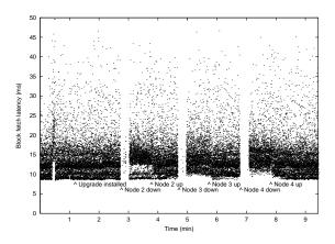
Fig. 4. DHash block fetch performance during an upgrade.
